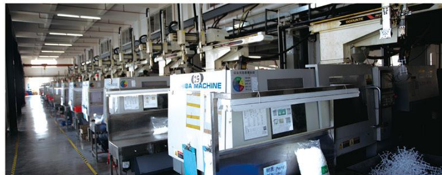
◆ 东芝注塑车间，全机械手自动化生产 Toshiba injection workshop; automatic production
