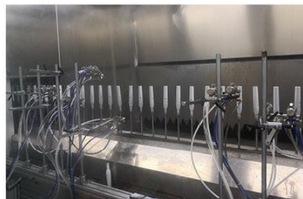
◆ 无尘自动喷涂车间：底油喷房 Dust-Free Plastic Automatic Spray Line: Undercoat Spray Area
