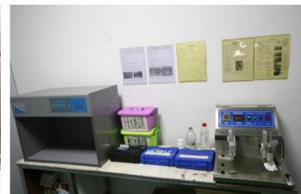
◆ 检测设备：耐摩擦试验机，灯箱，酒精 / 牙膏水 / 漱口水等化学试剂（根据客户产品要求） Test equipments: Friction testing machine, light box, Alcohol kit/ Toothpaste kit/ Mouth water kit (According product testing requirements)
