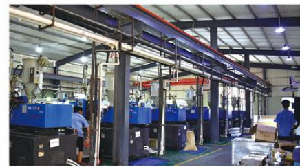
◆ 东芝注塑车间，全机械手自动化生产 Toshiba injection workshop; automatic production
